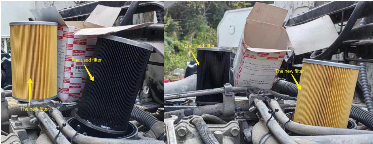
Engine diesel filter replacement
