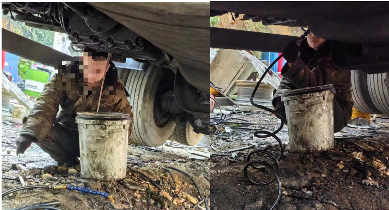
Transfer case gear oil replacement
